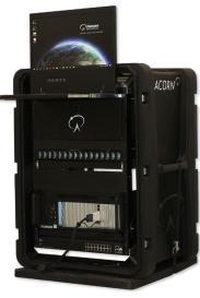
reconfigurable, closed-loop, end-to-end space system modeling and simulation environment that implements a Modular Open System Architecture (MOSA).
